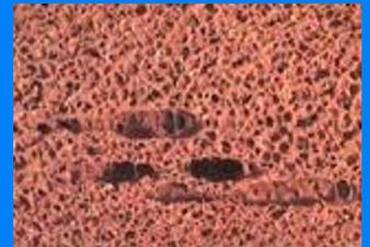
The inconsistency in the holes along a strip of rubber lead to varying degrees of recovery rate from the ejection material across the press, which in turn, means you have an unbalanced sheet.
