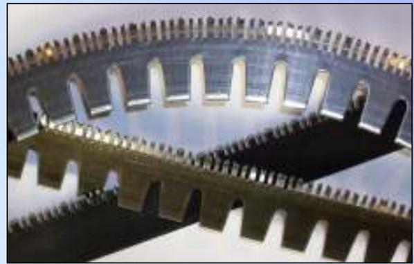
**SPEEDI~TEAR™** has applied scientific principles to each rule design to provide individual tooth and gap profiles to suit all corrugated flutes. These profiles are readily available for application with 2pt/3pt rules for flatbed die-cutting and 4pt rules for rotary conversion. 6pt rules are manufactured to order.
